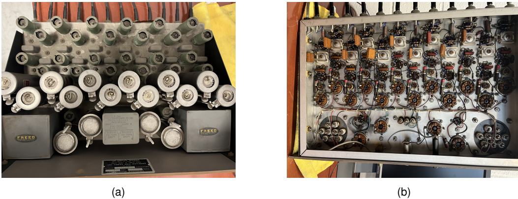
Figure 2: The top (a) and bottom (b) of the Tone Generator unit removed from the Mark II's rack. The tuning forks are housed in the twelve capsules along the center of (a).
